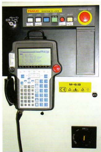
Obr. 6 Riadiaca jednotka Fanuc Robotics System R-J3iC Controller Fig. 6 Control unit Fanuc Robotics System R-J3iC Controller
